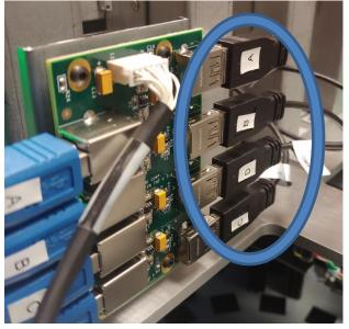
2. Remove the USB cable from the clip, and pull it through the zip tie that routes all of the USB recorder cables.
