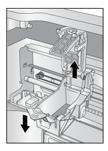
3. Remove the **All-in-One Ink Cartridge** from its packaging. Slowly remove the tape covering the cartridge's print head.
