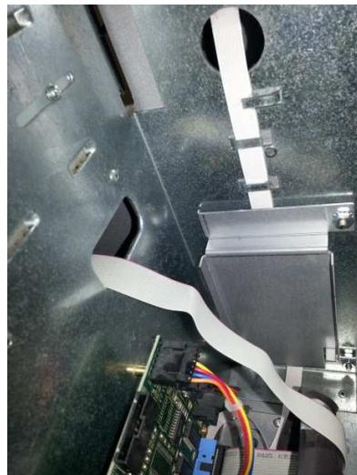
6. Install the power supply onto the bracket with the AC power connection facing up and ground prong facing away from the bracket. Secure the power supply using the **large tie wraps**.
