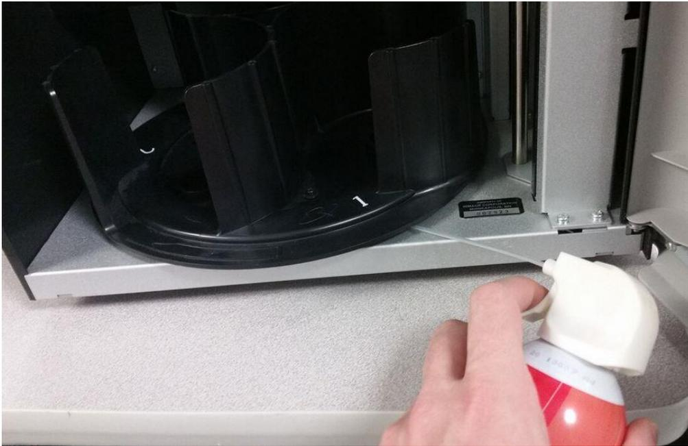
Tip: Focus on the 3'o clock position as this where the sensor is located.
