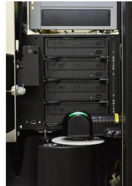
4. Manually, slightly rotate the **carousel** so that the distance between the edges of the carousel and the edge of the disc is equal on all four points, as shown.
