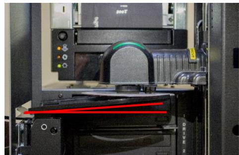
11. Position the **disc diverter** to the horizontal position.
