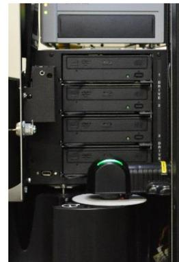
4. Manually, slightly rotate the **carousel** so that the distance between the edges of the carousel and the edge of the disc is equal on all four points, as shown.
