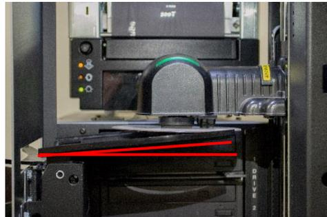
5. Position the **disc diverter** to the horizontal position.
