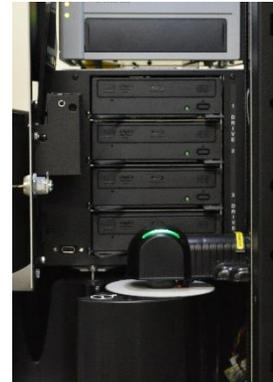
6. Manually, slightly rotate the **carousel** so that the distance between the edges of the carousel and the edge of the disc is equal on all four points, as shown.
