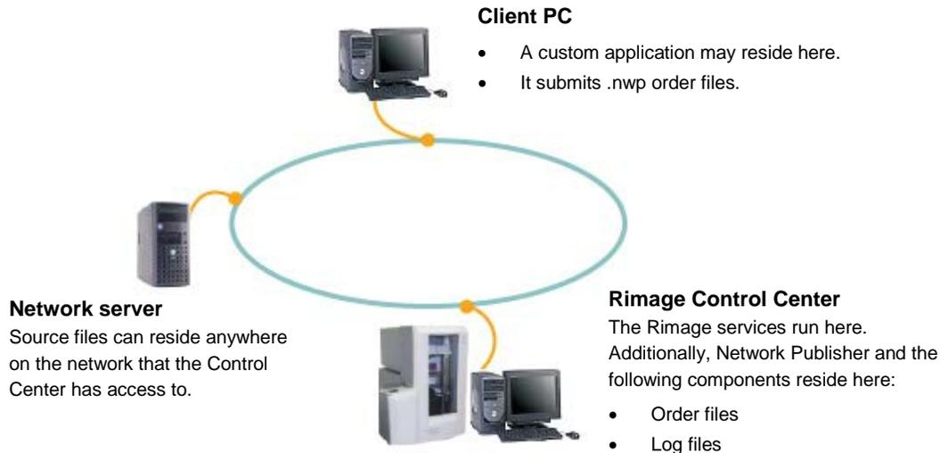
**Note:** Other network configurations are possible, for example the Network Publisher may be installed on a client PC, it does not have to run on the Control Center.
