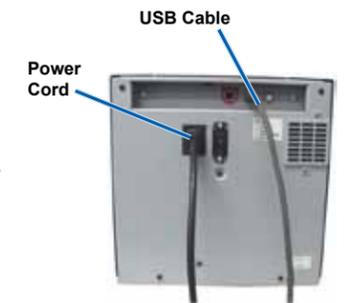
**Note:** The Everest printer powers on when the power cord is connected from the printer to the power outlet. You will be powering on the printer during driver installation in step 6.
