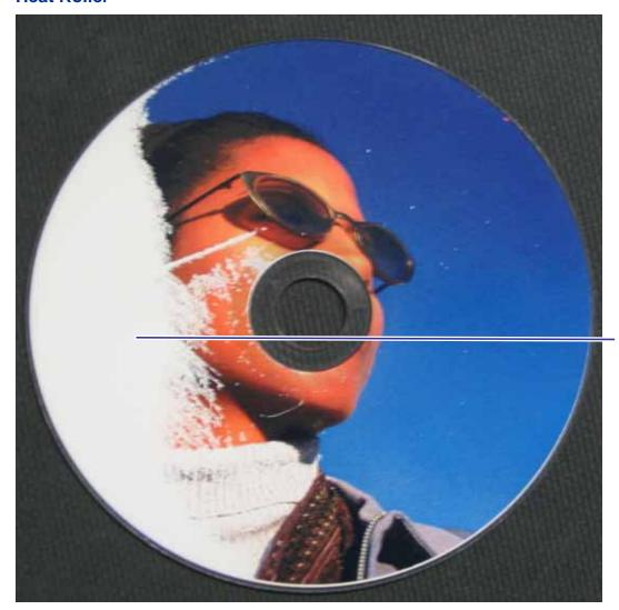
Narrow to wide vertical voids in the print on one side of the disk.
