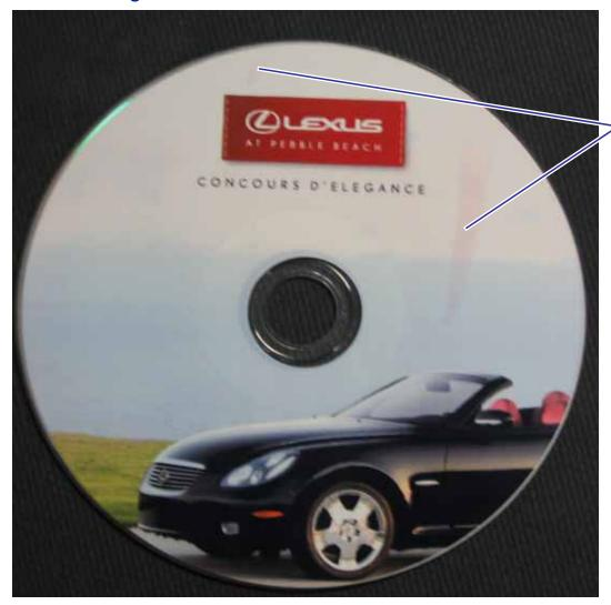
An area of shading or the wrong color embedded in the print
