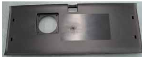
Item 8 – Rear Panel (see figure 2.8) Plastic may contain brominated flame retardants.
