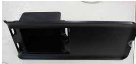
Item 3 – Side Panel (see figures 1.3 and 5.3 ) Plastic may contain brominated flame retardants
