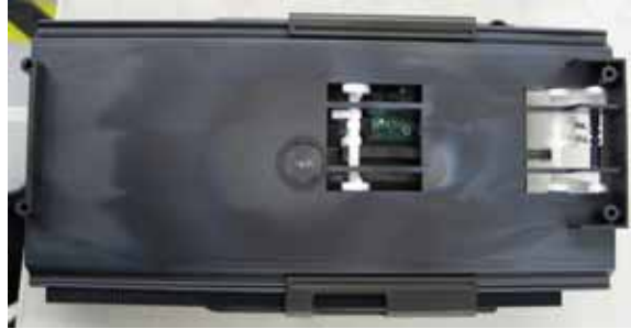
Item 6 – Printer Tray Assembly (see figure 1.6) Plastic may contain brominated flame retardants.
