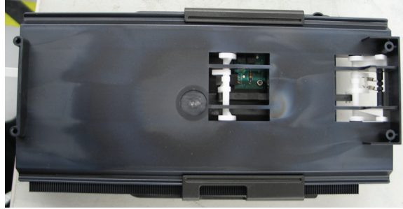
Item 20 – Printer Tray Assembly (see figure 7.20) Plastic may contain brominated flame retardants.
