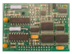
Item 15 – Piggyback board (see figure 10.15) Printed circuit board; pre-RoHS board may contain lead Boards marked with Pb-free symbol are RoHS compliant.
