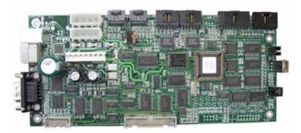
Item 11 – Control board (see figure 11.11) Printed circuit board; pre-RoHS board may contain lead Boards marked with Pb-free symbol are RoHS compliant.
