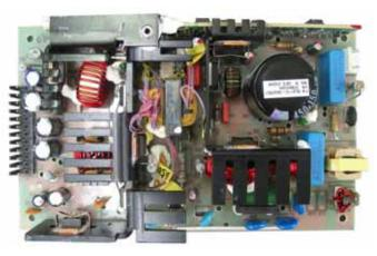
Item 13 – Power supply (see figure 11.13) OEM component; printed circuit board; pre-RoHS board may contain lead Boards marked with Pb-free symbol are RoHS compliant.
