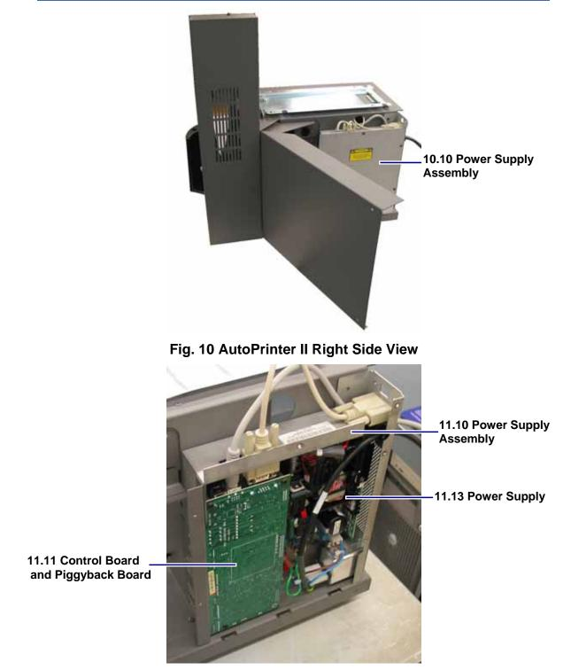
Fig. 11 Amigo II and AutoPrinter II Power Supply Assembly Interior View
