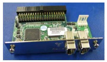
Item 5–Recorder Bridge Board (see figures 1.5 and 4.5) Printed circuit board; pre-RoHS board may contain lead. Boards marked with Pb-free symbol are RoHS compliant.
