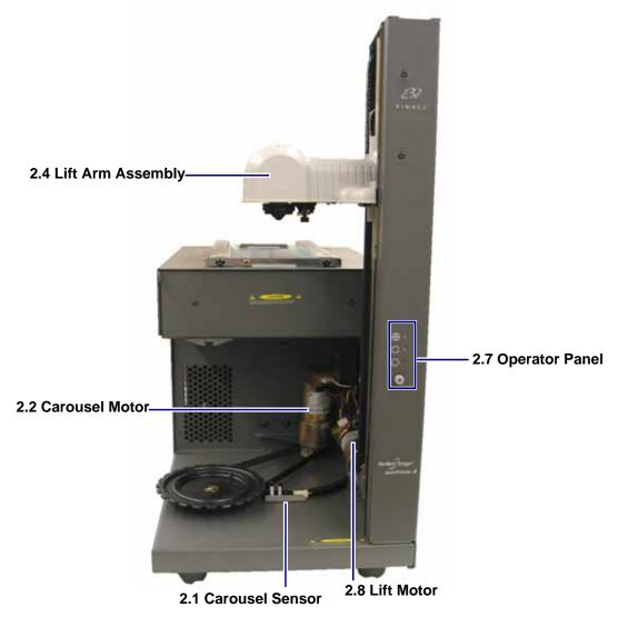
Fig. 2 AutoPrinter II Front View
