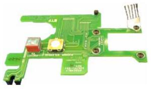
Item 4 – Lift Arm Control Board (see figure 1.4 and 2.4) Printed circuit board; pre-RoHS board may contain lead Boards marked with Pb-free symbol are RoHS compliant.
