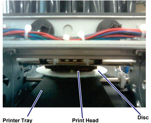
4. Run **diagnostic test 6** (print test) to check the print head alignment.
