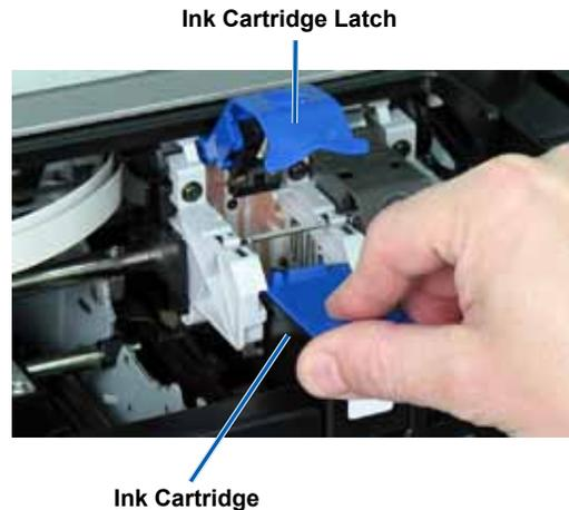
3. If an ink cartridge is already installed, slide the **ink cartridge** out of the ink cartridge cradle.
