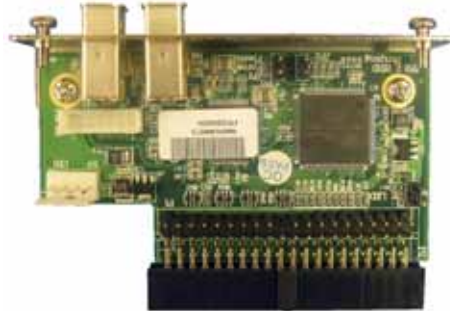
Item 7 – 1394b – ATAPI Bridge Board (see figures 2, 3 and 4)
