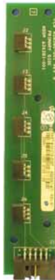
Item 2 – Collator Board (DLN5200 only) (see figure 1.2) Printed circuit board; pre-RoHS board may contain lead. Boards marked with Pb-free symbol are RoHS compliant.
