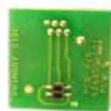
Item 2 – Collator sensor board (DLN5200 only) (see figure 1.2) Printed circuit board; pre-RoHS board may contain lead. Boards marked with Pb-free symbol are RoHS compliant.
