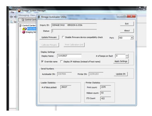
4. Select the firmware and press update firmware. When completed, restart the production server in Rimage System Manager.
