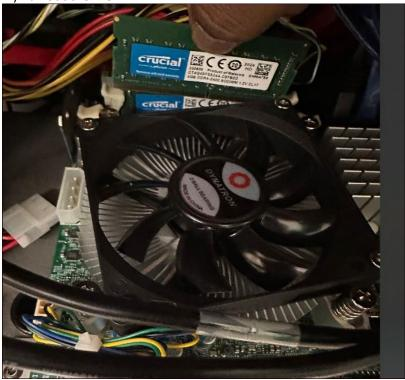
5.) Finally push the 8 GB RAM and lock the latch:
