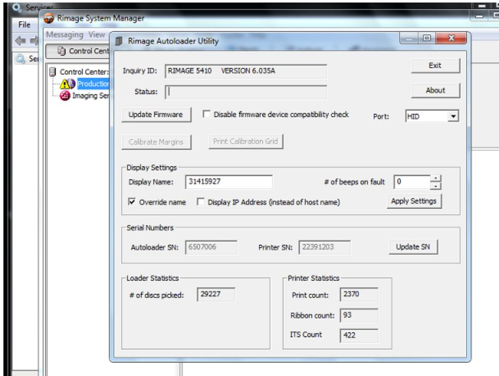
4. Select the firmware and press update firmware. When completed, restart the production server in Rimage System Manager.
