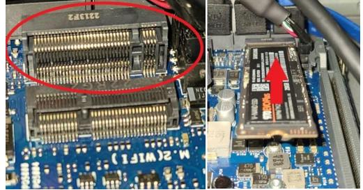
6. While holdind the drive down, fasten it in place with the screw removed in step 3
