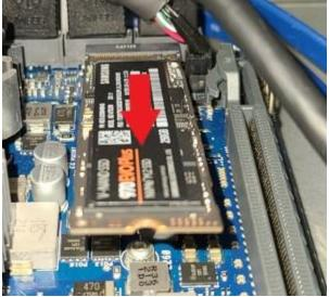
5. Insert the replacement M.2 drive into the top M.2 slot, with the notched to the right
