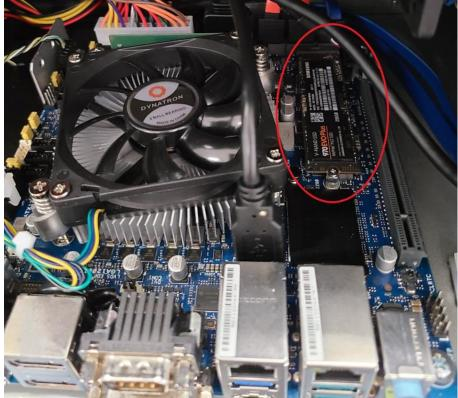
3. Remove the philip screw that holds the drive down.
