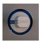
Mode 0 – Standalone mode. Use this mode for a standalone printer that is not connected to an autoloader. The printer will not attempt to communicate with an autoloader.
