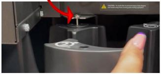
4. Rotate the carousel left and right to ensure it is properly seated. You should feel the resistance of the carousel motor.
