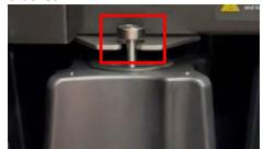
3. Move the carousel left and right, until it drops into the slots and the bearing drops into the bracket.
