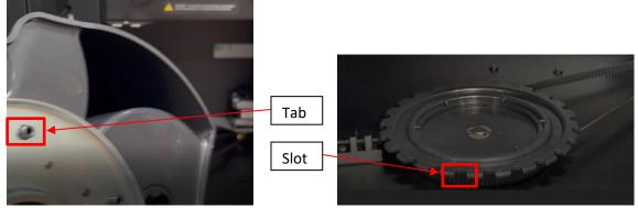
2. Place the carousel on the platter, lining up the tabs with the slots. Align the bearing with its bracket.
