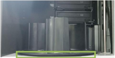
2. Blast compressed air into the gap under the carousel.
