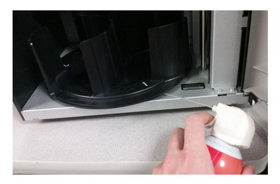
Tip: Focus on the 3'o clock position as this where the sensor is located.
