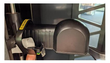
Push down on the front narrow end of the guard to secure its position.
