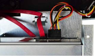
Disconnect the power cable and SATA cable from the back of the recorder that you wish to remove.
