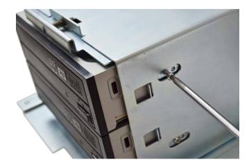
14. Close the **recorder bay**, setting it on the two **alignment pins** to properly align it with the undercarriage of the **Allegro 100** system.
