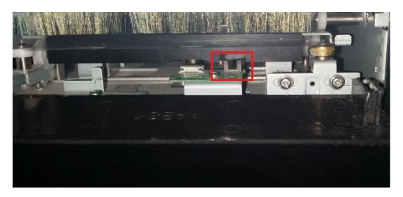
3. Unlock the flap. Firmly press down near the left hinge to unlock the flap.
